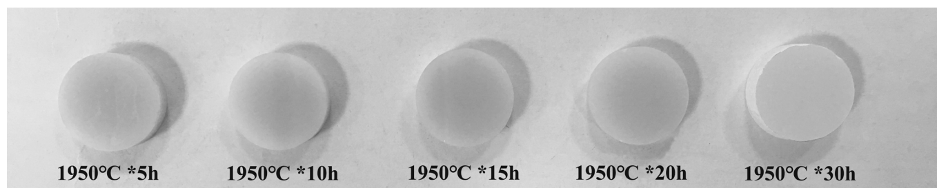
Fig. 6: Optical images of samples containing 30 mol% AlN – 70 mol% Al 2 O 3 after sintering at 1 950 °C for different holding times.
