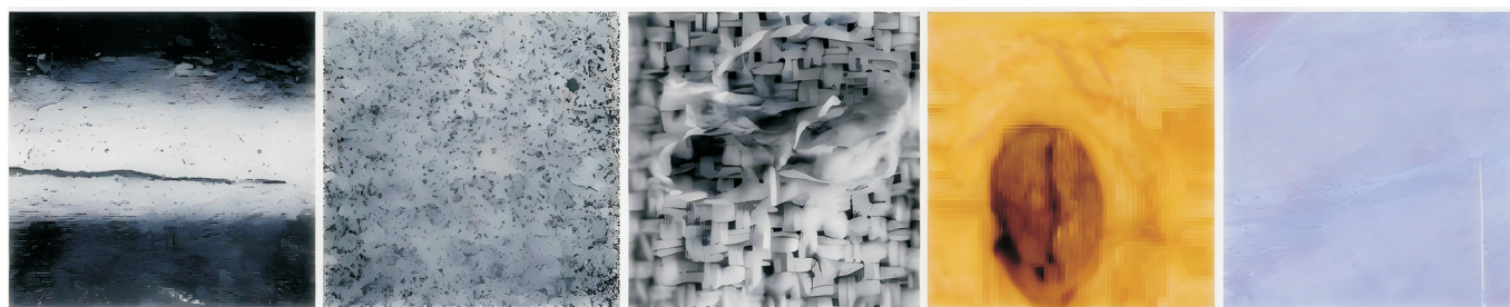
Fig. 2: Representative surface defects across various industrial materials. Illustrated from left to right are typical defect patterns observed on steel, stone, textile, wood, and ceramic tile surfaces. This comparison highlights the diversity of defect morphologies and textures that deep learning models must generalize across 28 .
