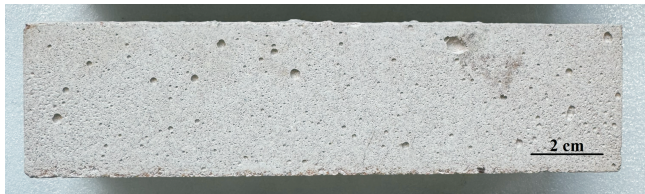
Fig. 10 . Lightweight castables specimen after two thermal shock cycles.
