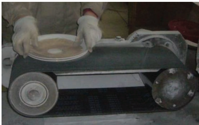
Fig. 2: Traditional way of grinding the bottom of ceramic plates.
