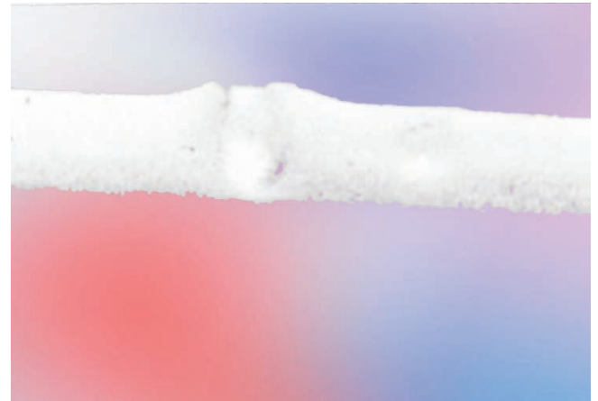
Fig. 2: Case 2 Cross-section of a pinhole.
