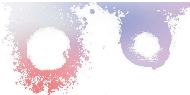
Fig. 1: Case 1 Cross-section of a pinhole.
