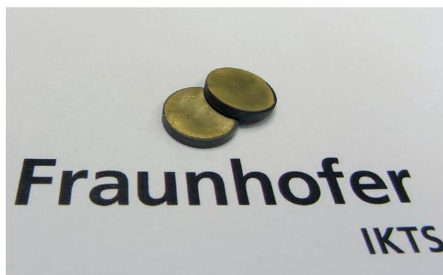
**Fig. 9:** Successful metallization of gold on C12A7:e<sup>-</sup> ceramic.
