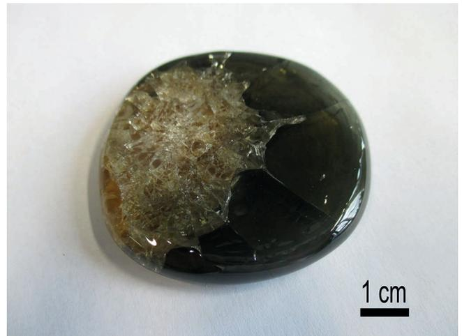
Fig. 1: Cracked glass-ceramic disc of C12A7 composition after melting and quenching.
