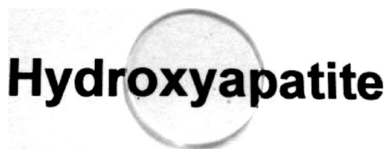
Fig. 4: Transparent hydroxyapatite bioceramics prepared by spark plasma sintering at 900 °C from nano-sized HA single crystals. Reprinted from Ref. 112 with permission.
