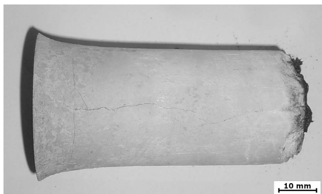
Fig. 2: Zirconia material N6 after the corrosion test for 6.5 hours.
