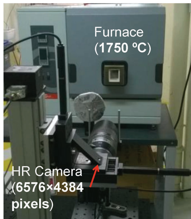
Fig. 1: Photo showing the in-situ measurement device.
