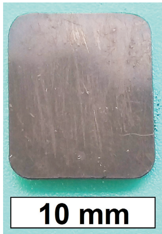
Fig. 7: WC-Co test sample 2 manufactured with T3DP – back.
