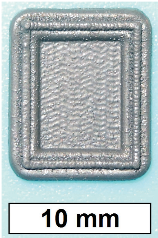
Fig. 6: WC-Co test sample 2 manufactured with T3DP – top view.
