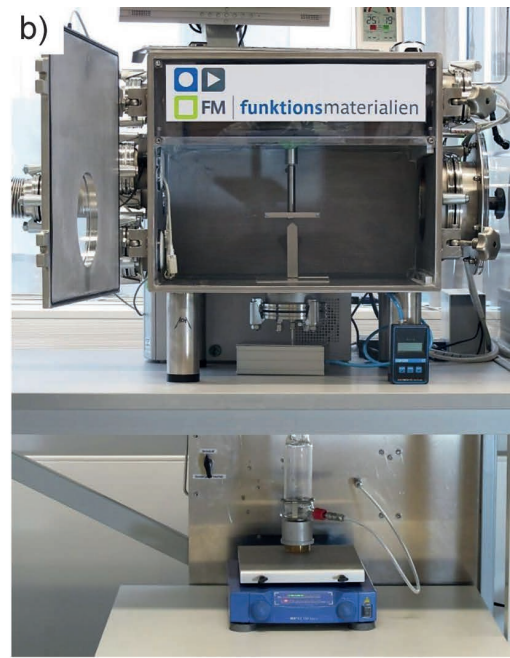
Fig. 3: (a) General schematic diagram of an AD setup (modified after 13 ) and (b) photo of an aerosol generation unit and AD chamber at the Department of Functional Materials at the University of Bayreuth.
