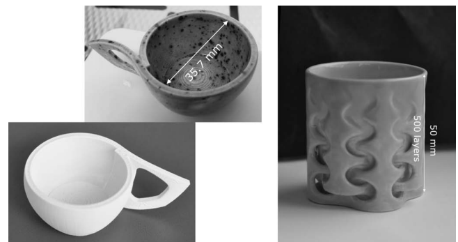
Fig. 4: Lower left, biscuit-fired cup, upper left, glazed and glost-fired cup from Fig. 3, right, glazed and glost-fired cup. All cups shown are made of porcelain with the application of the LSD technology.
