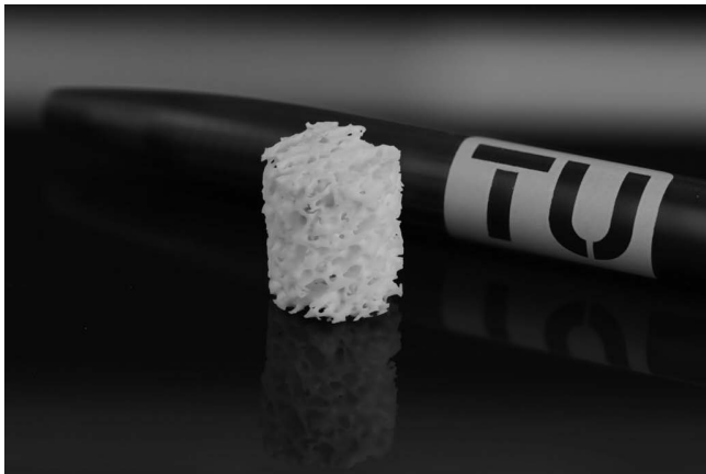
Fig. 1: Trabecular bone scaffold made of 45S5 Bioglass® and additively manufactured by the SLCM process (10 mm in diameter, 10 mm high); the geometry was generated using \mu CT images of human femoral bone (pen to scale); Vienna University of Technology.
