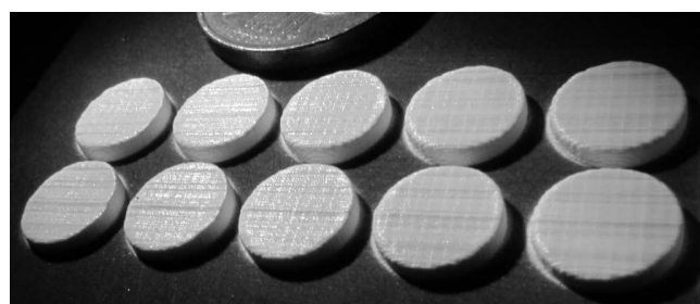
Fig. 7: Green Al 2 O 3 -3Y-TZP cylinders consisting of 800 layers.
