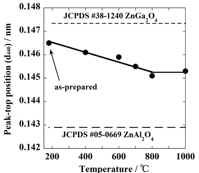
Fig.10: Peak-top position ( $d_{440}$ ) of cubic spinel phase of samples hydrothermally formed at 180 °C before and after heating at 400 ~ 1000 °C for 1 h.
