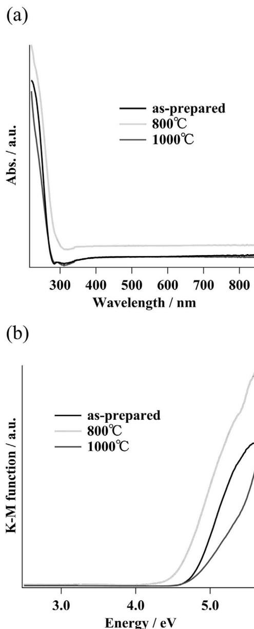
**Fig. 11:** (a) Diffuse reflectance spectra of samples hydrothermally formed at 180 °C before and after heating at 1000 °C for 1 h. (b) Plots of transformed Kubelka-Munk function vs. the energy of light absorbed of samples.
