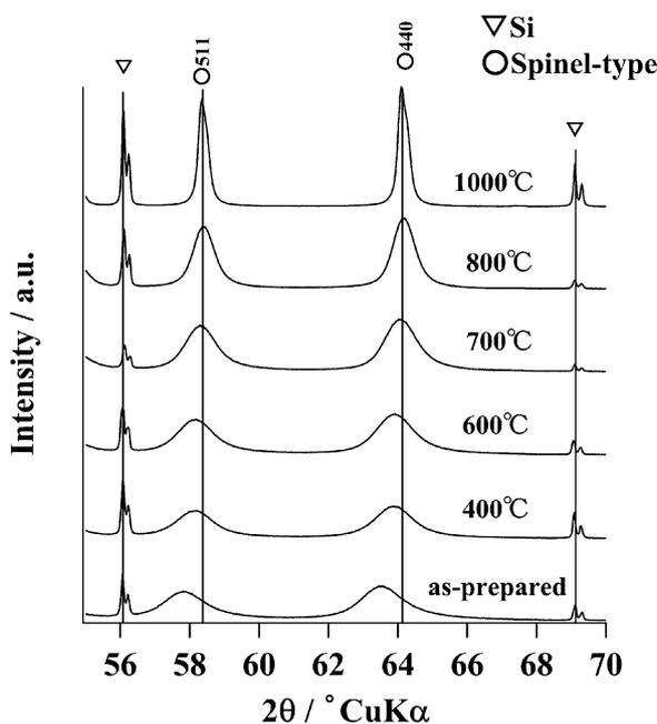
Fig. 9: Close-up of the region around 58 ~ 64 °; 2θ of the x-ray diffraction patterns of samples hydrothermally formed at 180 °C before and after heating at 400 ~ 1000 °C for 1 h.
