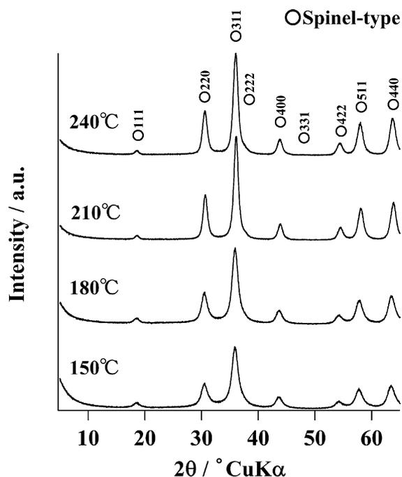
Fig. 1: X-ray diffraction patterns of precipitates obtained under hydrothermal conditions at 150 ~ 240 °C for 5 h.
