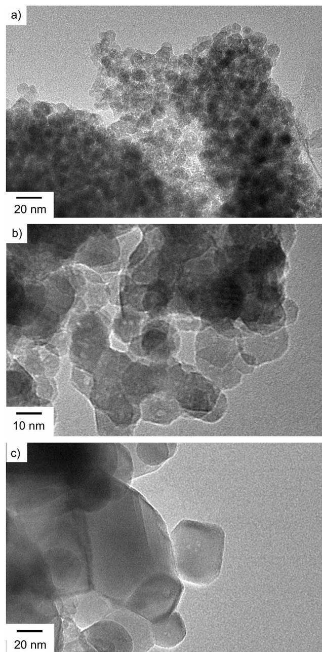
Fig. 6: Transmission electron microscopy images of samples heated at (a)  $600^\circ\text{C}$ , (b)  $800^\circ\text{C}$ , and (c)  $1000^\circ\text{C}$  for 1 h.
