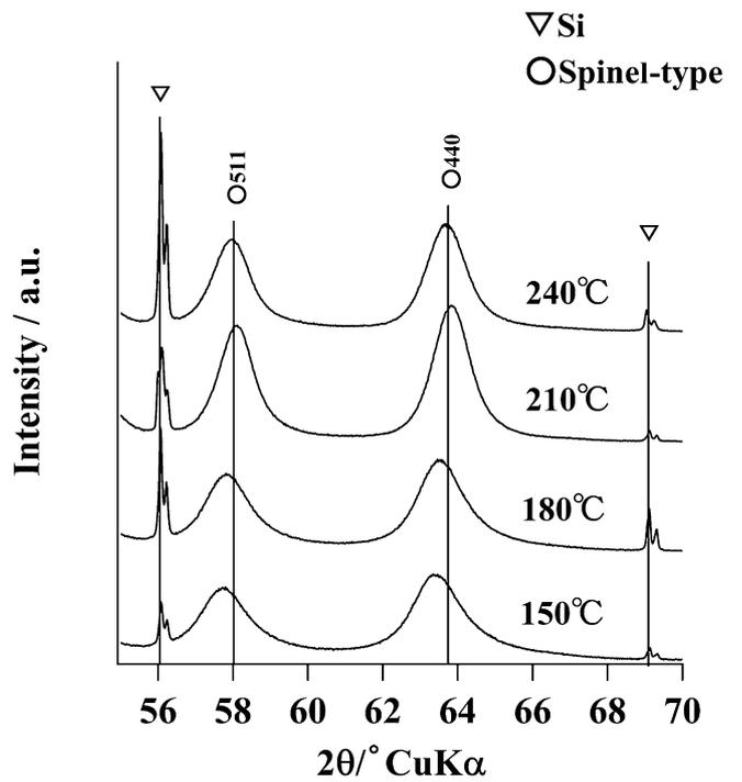
Fig. 3: Close-up of the region around 58 ~ 64° 2θ of the x-ray diffraction patterns of samples obtained under hydrothermal conditions at 150 ~ 240 °C for 5 h.
