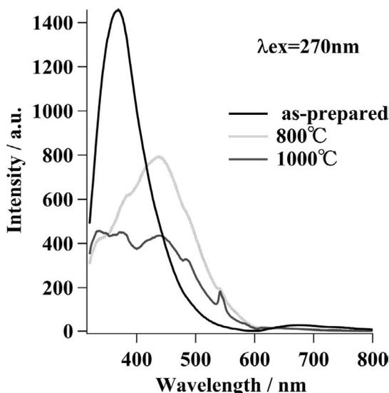
Fig. 12: Emission spectra of samples as-prepared at 180 °C and after heating at 800 and 1000 °C for 1 h. ( $\lambda_{\text{ex}} = 270$  nm)
