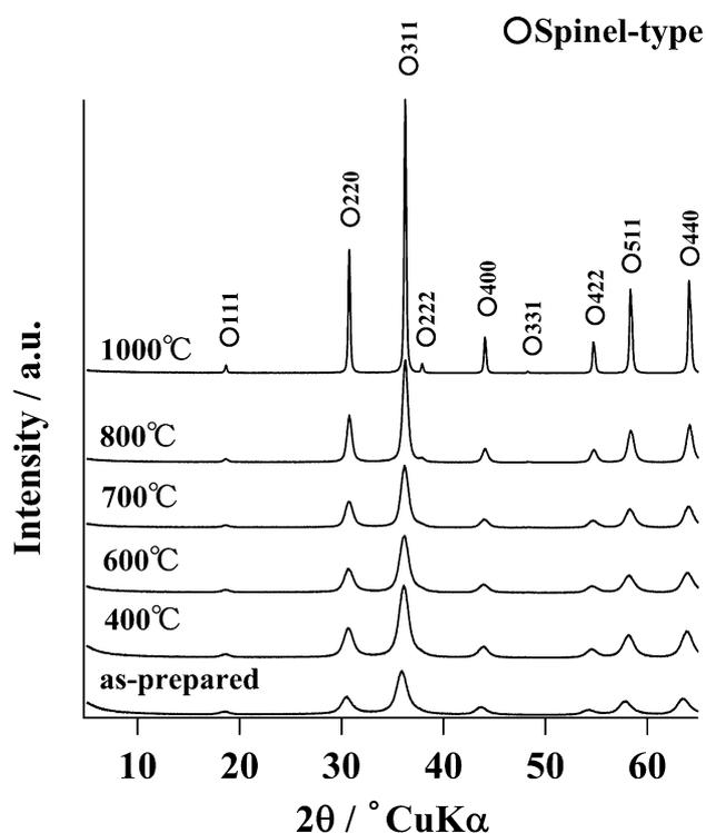
Fig. 5: X-ray diffraction patterns of samples hydrothermally formed at  $180^\circ\text{C}$  before and after heating at  $400 \sim 1000^\circ\text{C}$  for 1 h.
