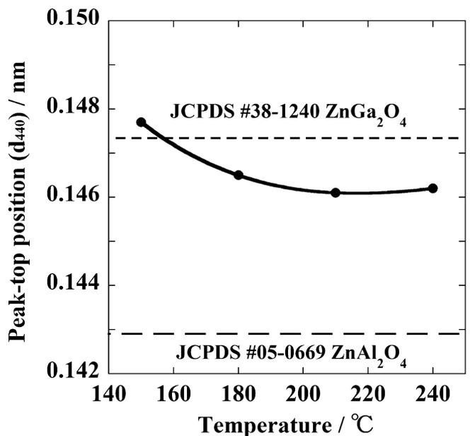
Fig. 4: Peak-top position ( $d_{440}$ ) of cubic spinel phase of samples obtained under hydrothermal conditions at 150 ~ 240 °C for 5 h.
