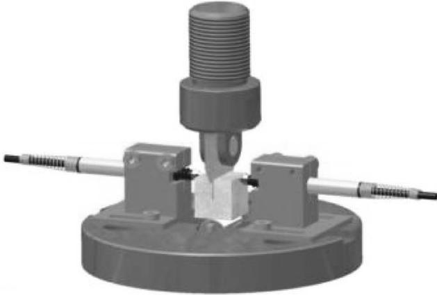
Fig. 1b: Experimental set-up for WST at RT.
