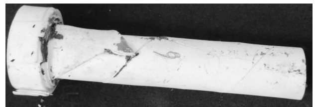
Fig. 9: Complete nozzle after six thermal shocks in tin melt (500 °C); all visible cracks were already formed during sintering.
