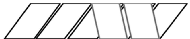
Fig. 1: Scheme of the spiral winding technique (dark: first layer; light: second layer, rotated by 90° to the previous layer).
