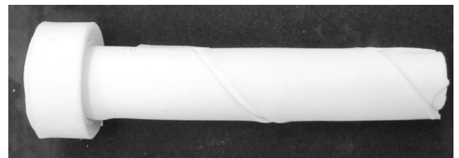
Fig. 2: Sintered nozzle with a fixture after removal of the outer layer (tube length: ~ 80 mm).
