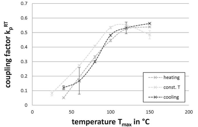
Fig. 1: Planar coupling factor of PIC181 as a function of temperature  $T_{\max}$  for different poling paths.
