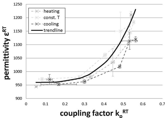
Fig. 2: Relative permittivity of PIC181 over coupling factor  $k_p^{RT}$  for different poling paths.
