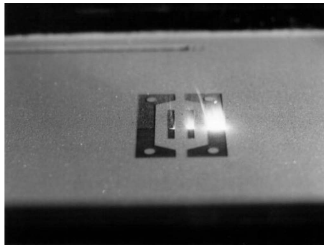
Fig. 8: SiSiC mirror with inner cooling channels during laser sintering.
