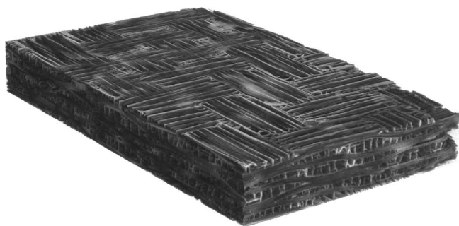
Fig. 10: A 3-D image reconstruction of a porous Si-SiC ceramic using computed tomography (novolac resin, twill-weave-derived).
