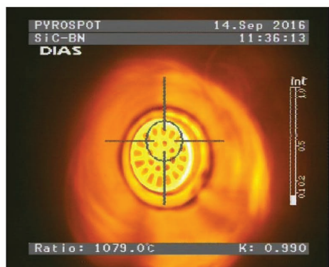
Fig. 10: Top: The solution adopted enhances heat exchange with engineered porous architectures. Bottom: Camera view of the inside of the tube during preliminary tests in a high-temperature experimental apparatus. The image shows the inlet of the tube with an air mass flow of 5 \text{ g}\cdot\text{sec}^{-1} while the outer tube walls are kept at 1280^\circ\text{C} .
